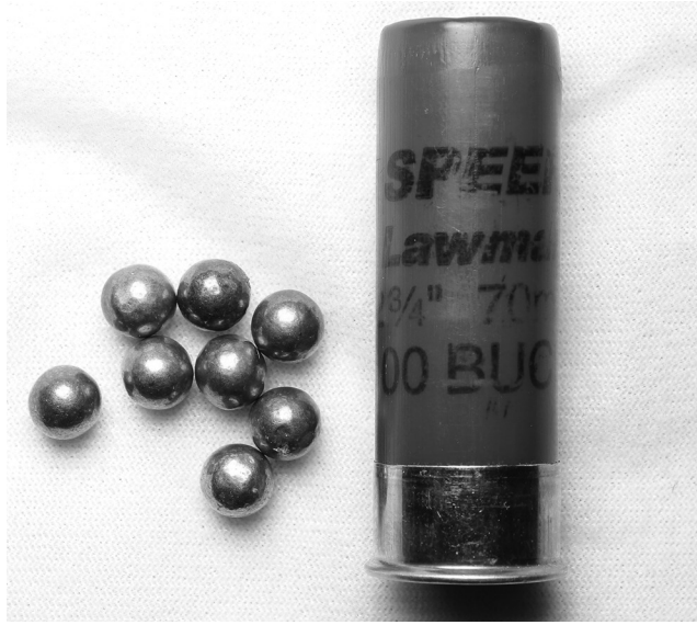
Figure 2.32 Speer Lawman 12-gauge shot shell loaded with 00 buckshot. This particular load uses eight copper-coated pellets instead of the more traditional nine-pellet load that has been preferred by the industry. (Image from author's collection.)
